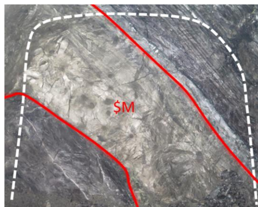
445 ore drive (4.5m W x 4.5m H) with a face grade of 5.5% Ni
