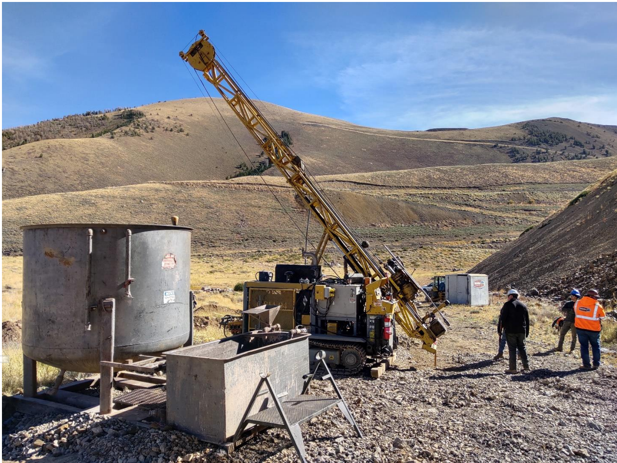
Figure 4: Diamond rig setting up on the drill pad for hole ZBF003 at South Sammy
