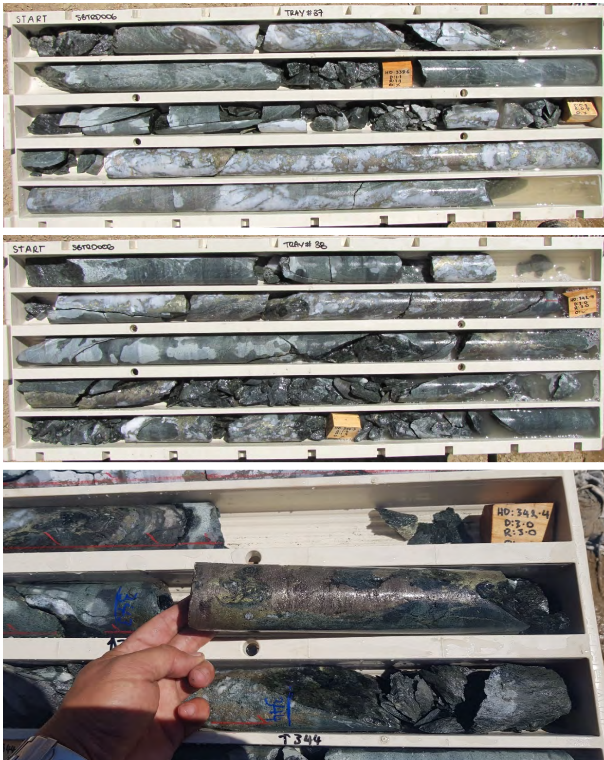
Figure 18. Bottletree SBTRD006 core: Top and middle photographs showing Trays 37 and 38 containing drill core from down hole depths 337m – 341.5m (approx.) and 341m – 344.5m (approx.) respectively, showing strong chalcopyrite and pyrite mineralisation. Bottom photograph shows close-up view of drill core from 343m (approx.).
