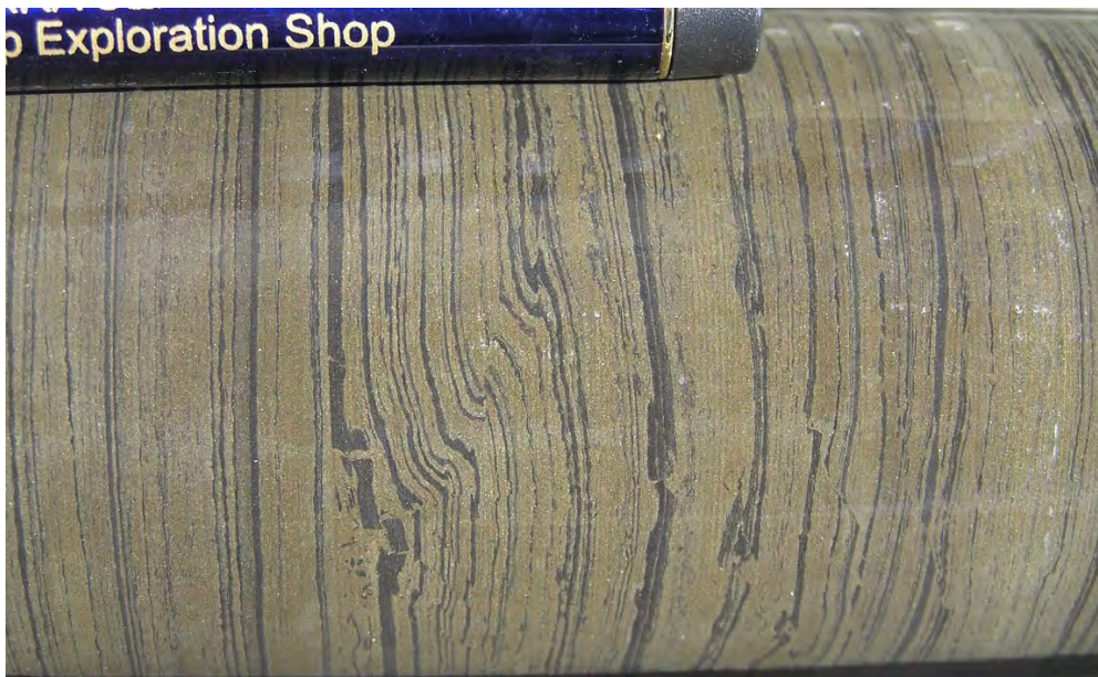
Figure 27. Well-developed stratiform pyritic shale intersected within Mount Les Siltstone from historical drilling of the Walford South VTEM anomaly by Superior Resources Limited.
