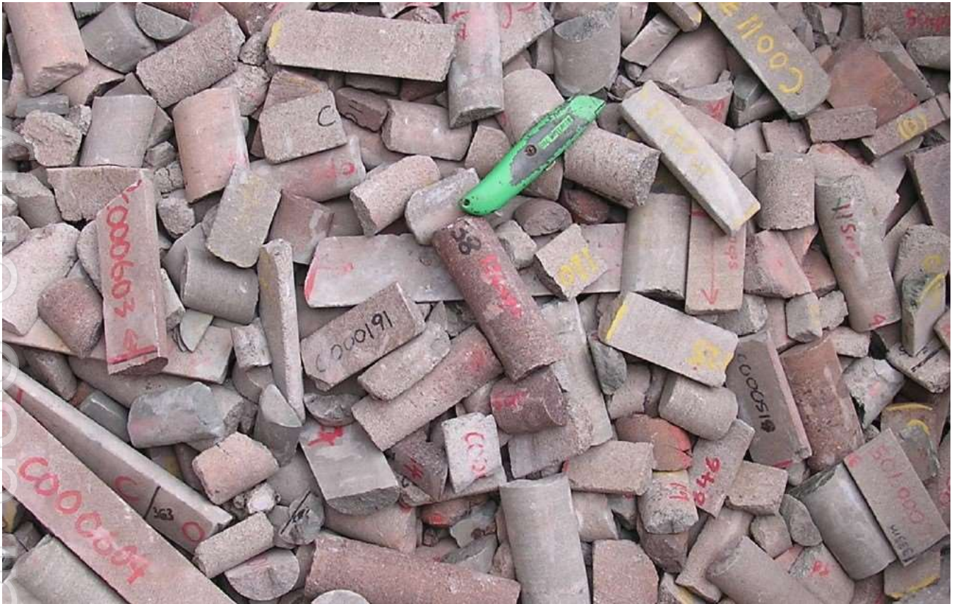
Figure 3 – Photo of NQ Core Used in Testwork Program
