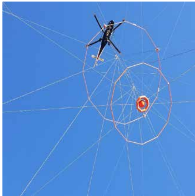
Photo 5 - VTEM Plus™ Survey being undertaken at Oracle Ridge
