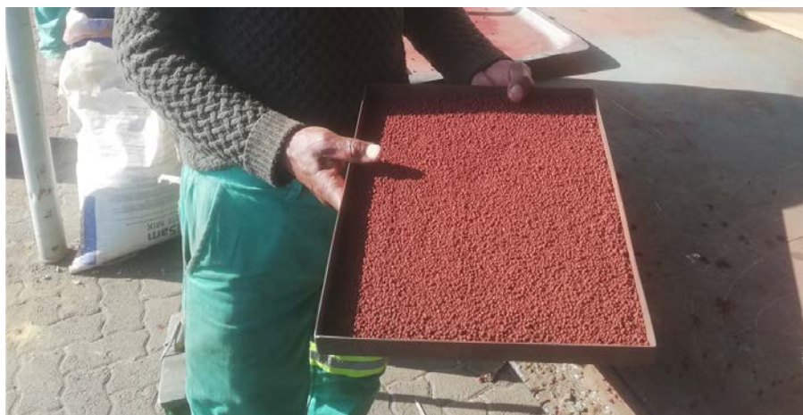
Figure 3: Agglomeration of iron fines into pellets
