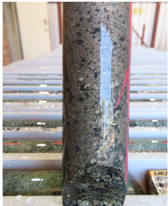
Figure 1: Massive, semi-massive and blebby nickel and copper sulphides in ANDD0003: ~79m downhole
