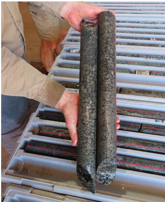
Figure 1: Massive, semi-massive and blebby nickel and copper sulphides in ANDD0003: ~79m downhole
