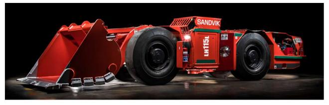
Sandvick low Profile LHD – At a height 1.6 m designed for operation in narrow-reef drill drives
