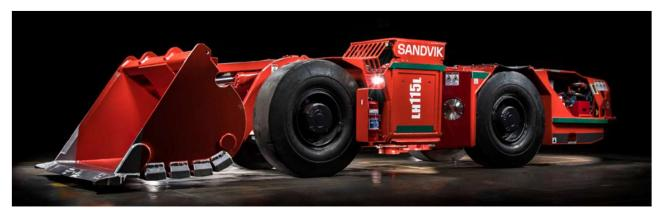
Sandvick low Profile LHD – At a height 1.6 m designed for operation in narrow-reef drill drives
