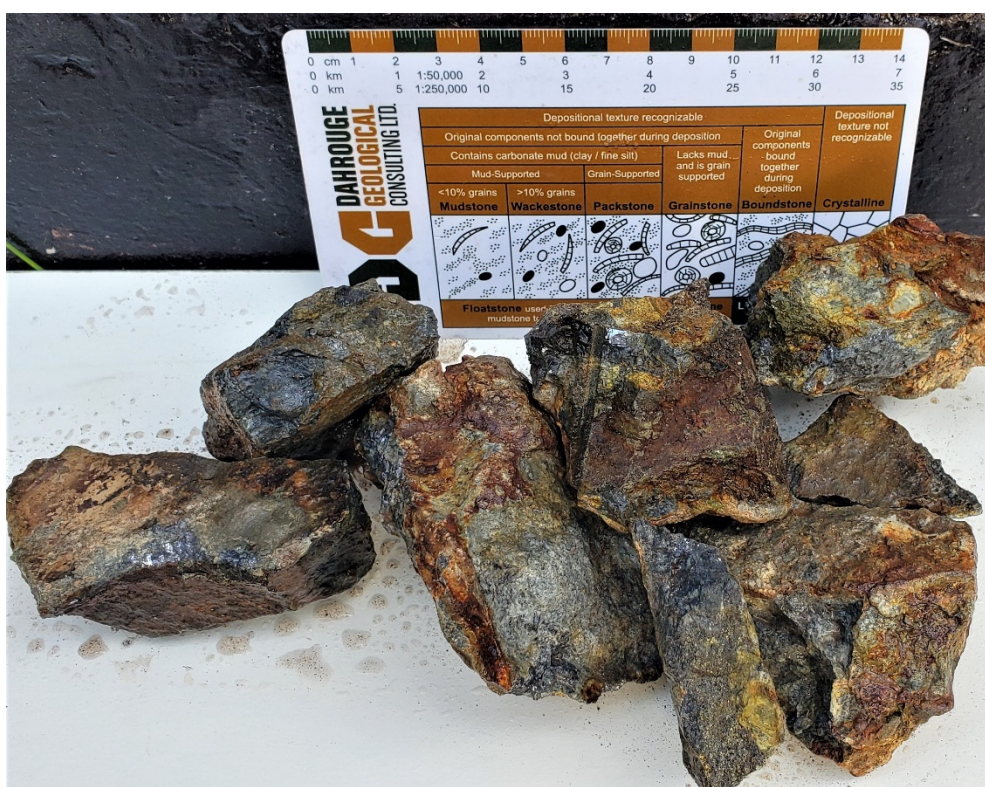
FIGURE 1: 35.4% Pb, 5.4% Zn, 2.24% Cu, >100g/t Ag
