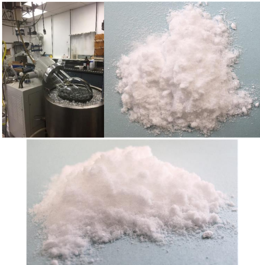
Figure 1: Hazen Research – Neutralisation and precipitation of Lake’s lithium product at its lab in Colorado, USA, with the production of Lake’s lithium carbonate product.
