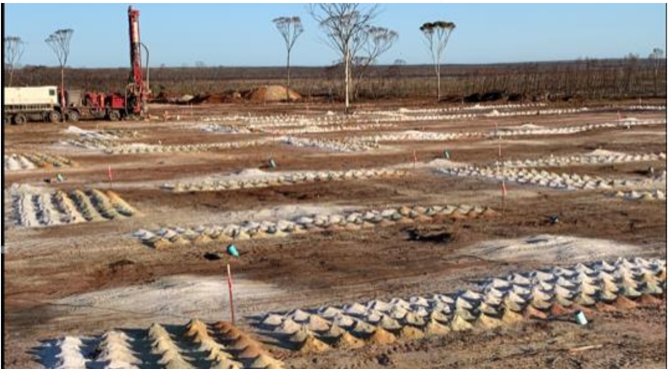
Figure 2: Infill RC drilling at Kat Gap
