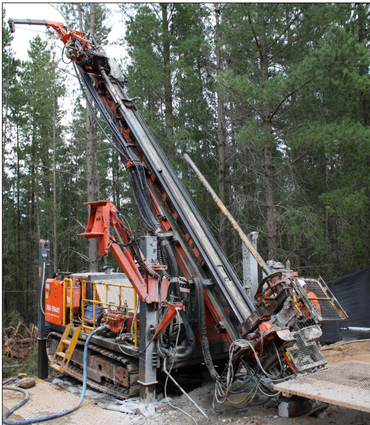
Figure 1: Diamond drill rig in operation at the Lightning Prospect, Castlemaine Gold Project (EL006679)
