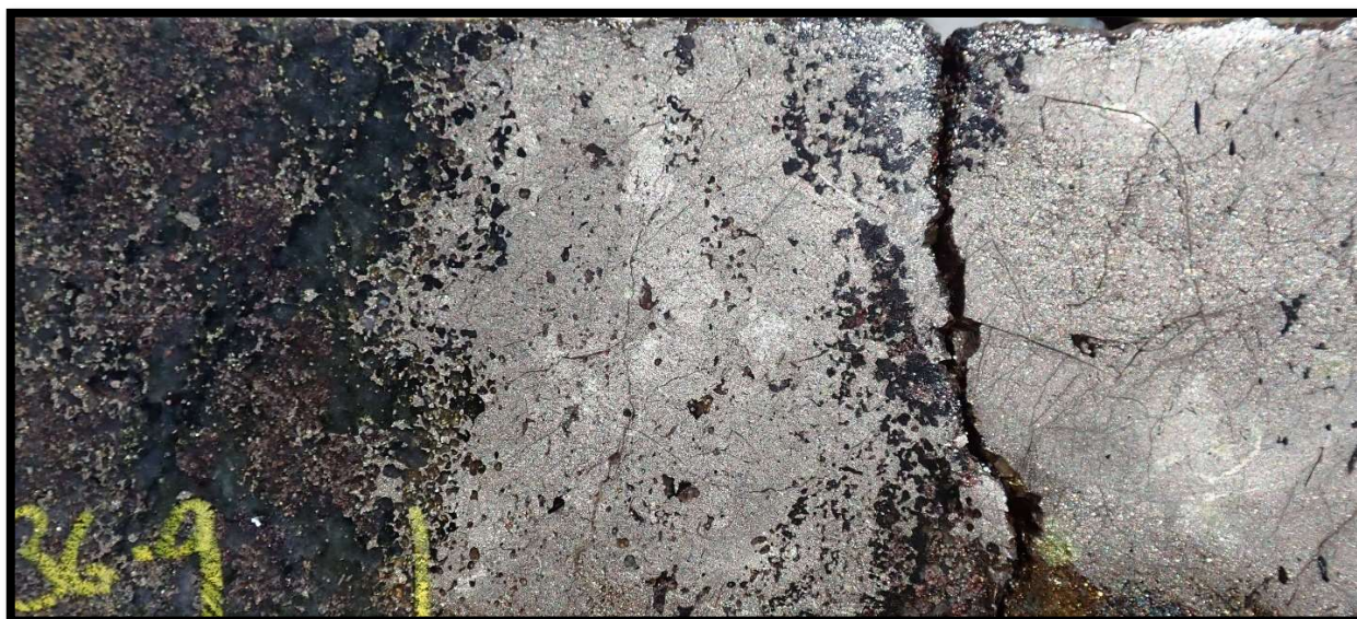
Melting Texture of Semi-Massive Ni-Cu Sulphide instead of Extension Veins from RKDD023 from 236m, NQ2
