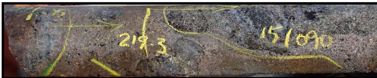
Melt Migration Texture of Massive Ni-Cu Sulphide from RKDD023 from 219m, NQ2
