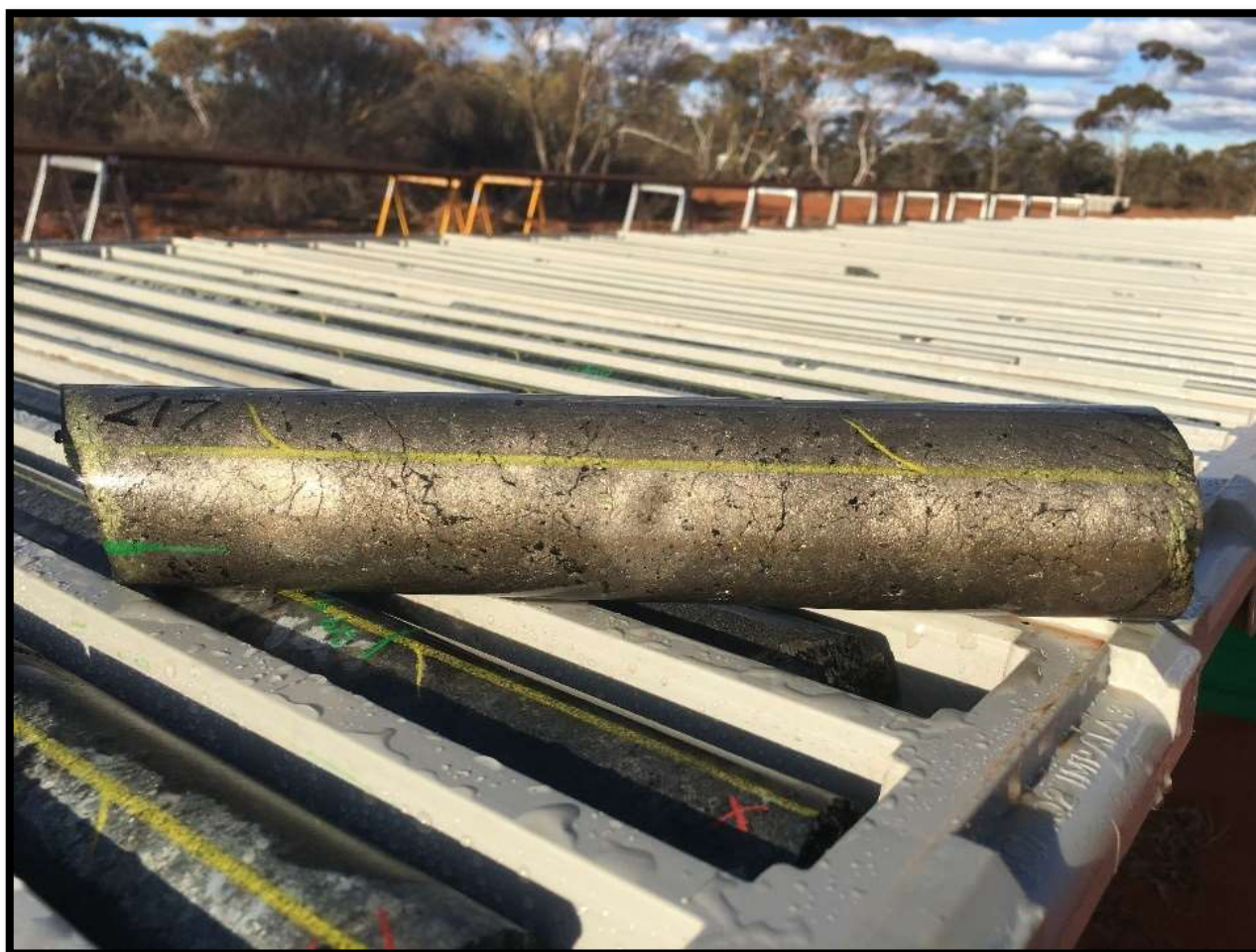
RKDD025 Massive Ni-Cu Sulphide from 217m, NQ2
