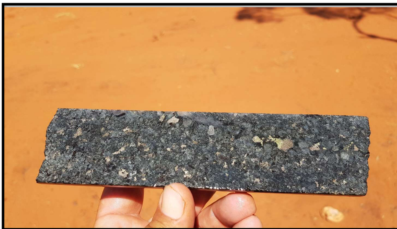
RKDD024 Disseminated and Blebby Ni-Cu Sulphide from 118m, NQ2
