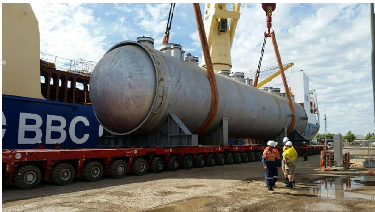
Figure 5: Sunrise Autoclaves Being Unloaded at Port Pirie
