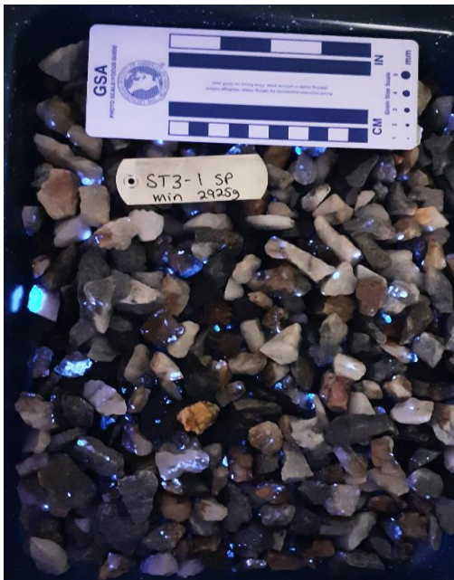
Figure 1 - XRT Sorter Product with scheelite under ultraviolet lamp
