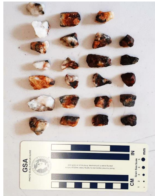
Figure 2 - XRT Sorter Product with high-grade wolframite particles
