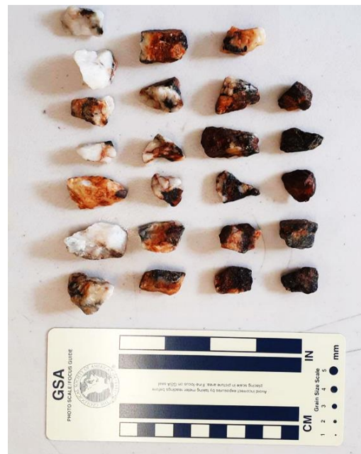
Figure 2 - XRT Sorter Product with high-grade wolframite particles
