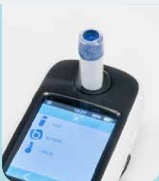
Senses temperature and reads ID through frost
