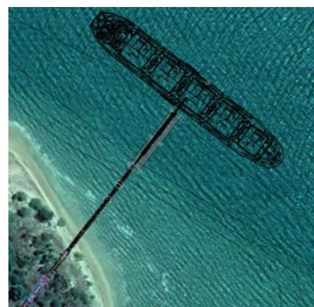
Figure 7 – Plan view of shiploader design and graphic moored ship envisaged for Option 1 and 2
