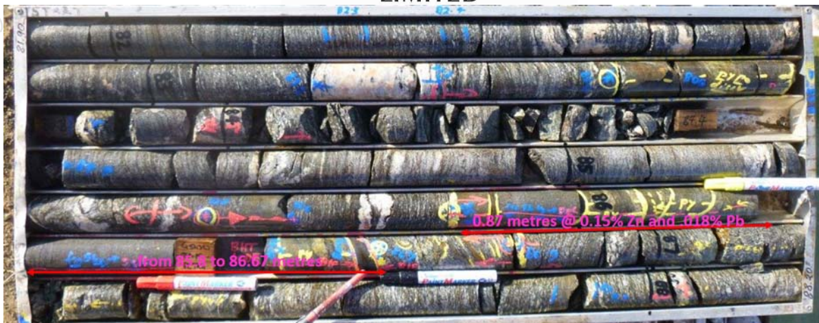
Figure 6: Mineralised garnetite & BIF bearing BHT Lode Zone 2 from 85.5 to 86.9 m within a larger interval of anomalous zinc.
