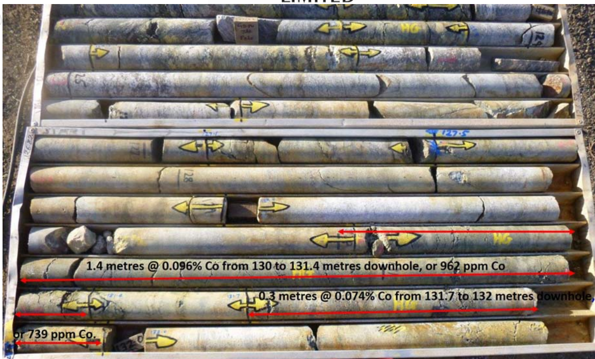
Figure 4: Pyrite zone in DD95STV3 from around 123 to 133 m relogged.
