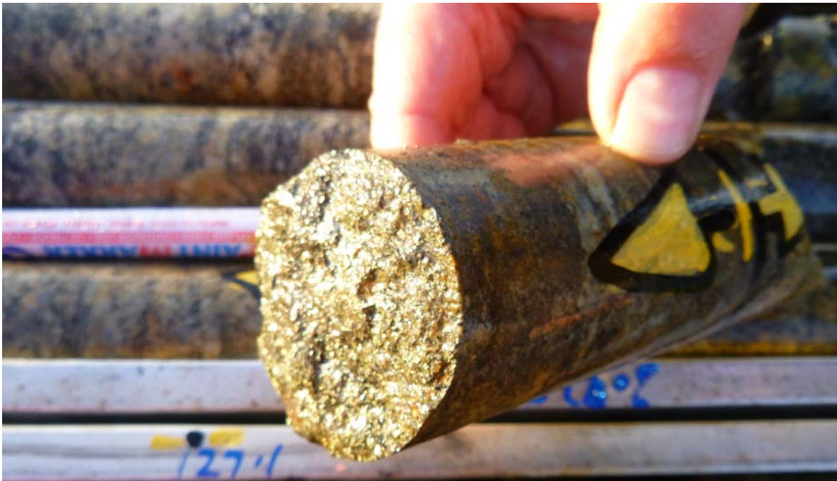
Figure 3: An example of the strongly pyritic bands in albitic gneiss in DD95STV3.
