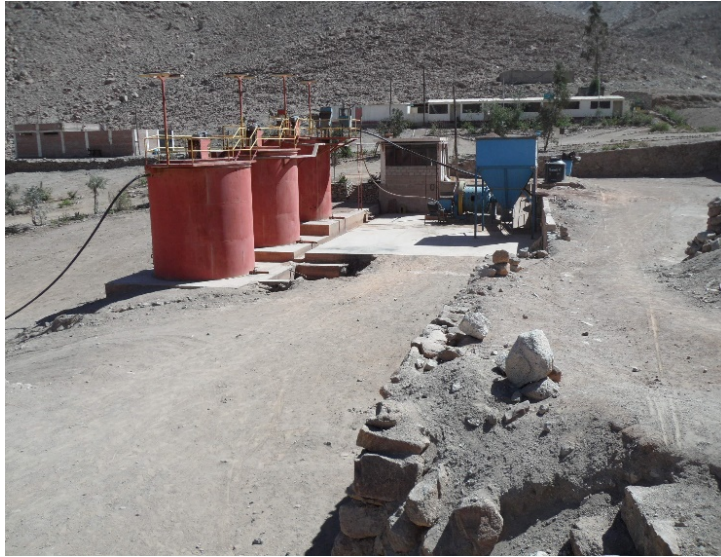
Figure 16: “Existing leach tanks: with accommodation block at rear left & Laboratory in the background: Chimú Gold Plant”
