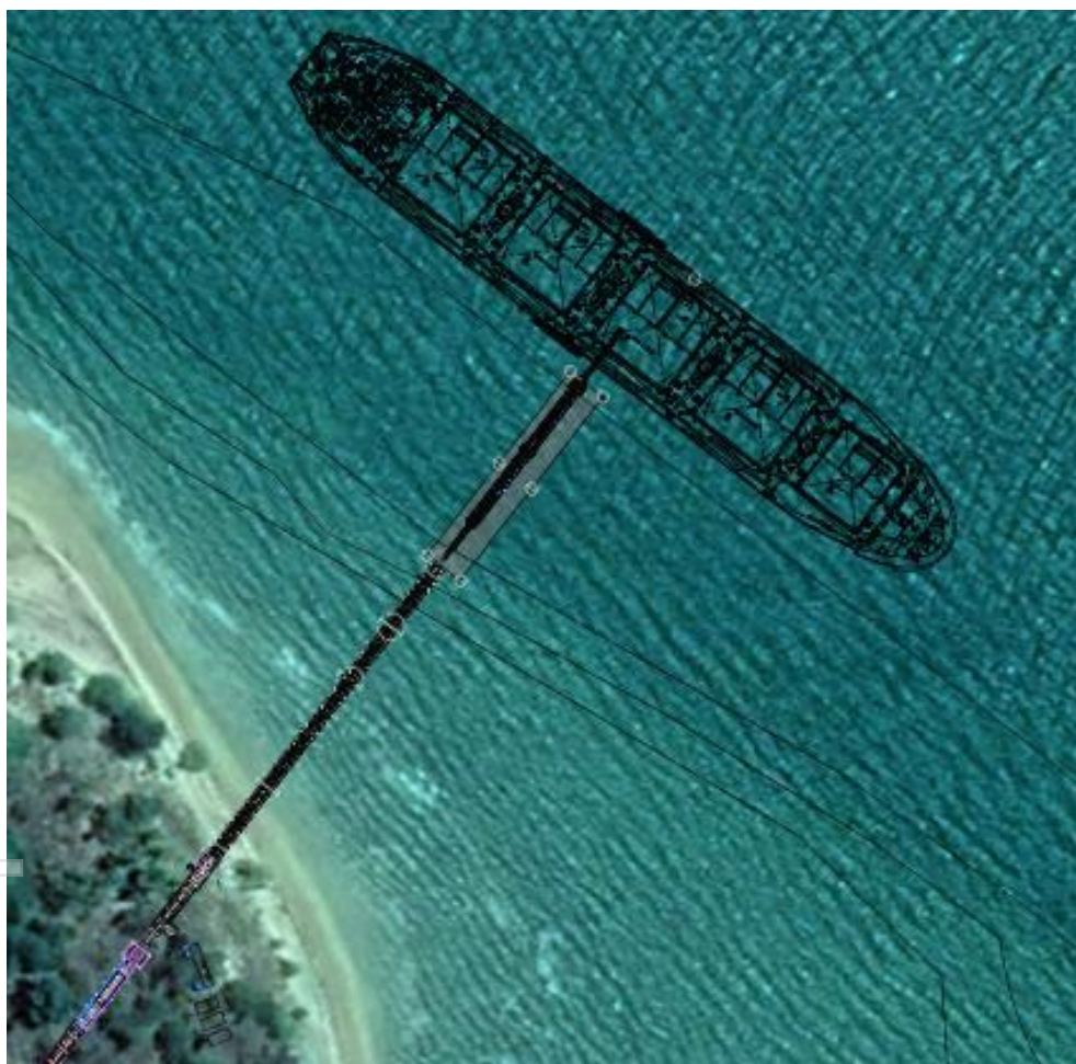
Figure 4: Plan view of shiploader design and graphic moored ship envisaged for Option 1 and 2
