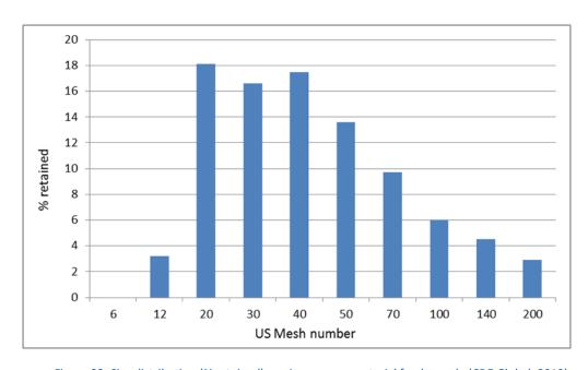
Figure 32: Size distribution (% retained) on sieves – raw material feed sample (CDE Global, 2019)
