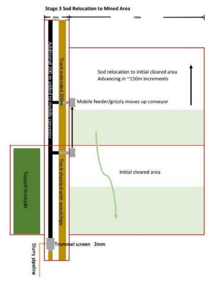
Figure 21: Mining process – silica sand mined in 2.25 ha panels
