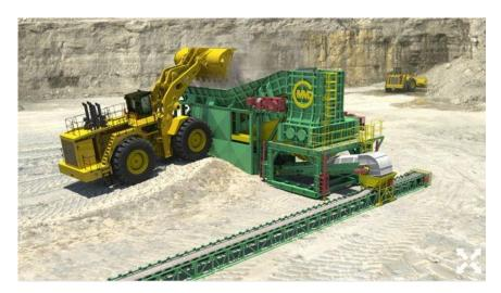
Figure 23: Mining process – silica sand loaded and screened
