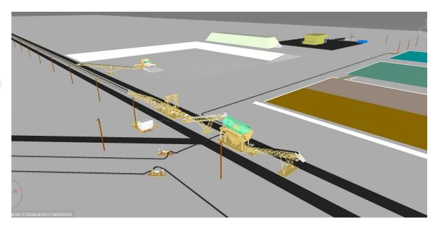
Figure 46: Feeder and Trommel Arrangement
