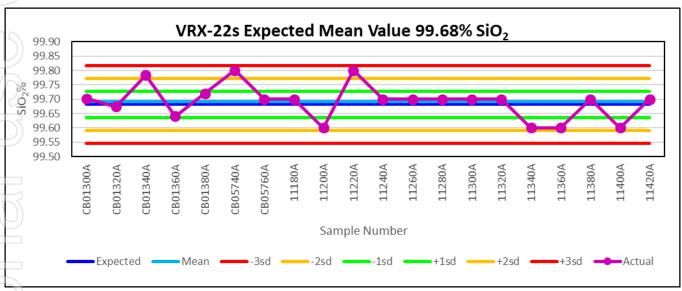
Figure 6: Control Chart for VRX-22S - SiO<sub>2</sub>
