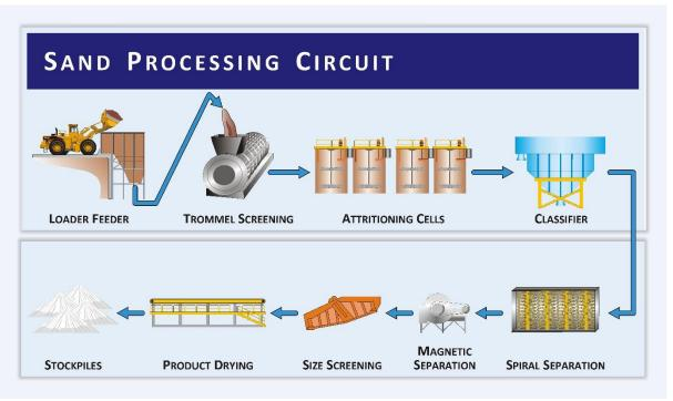
Figure 47: Sand Processing Circuit
