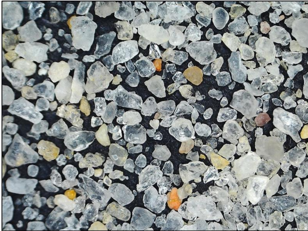
Figure 33: Arrowsmith Central sand (0.212-0.425 mm non-magnetic fraction Sphericity = 0.6 and roundness = 0.4)
