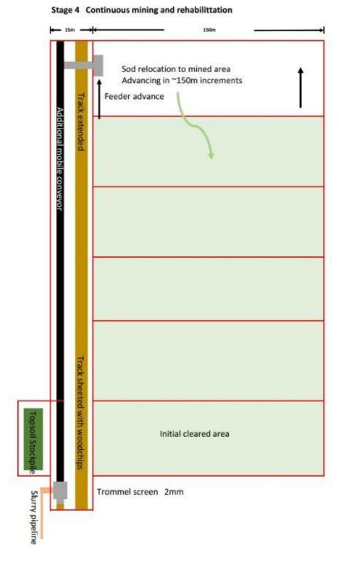
Figure 22: Mining process – continuous process of mining and rehabilitation
