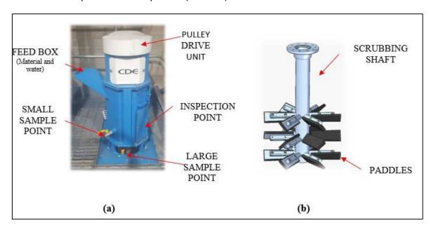
Figure 27: Lab scale attrition mill (left) and paddle shaft from lab scale attrition mill (right)
