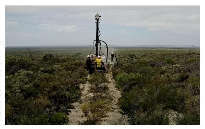
Figure 4: Landcruiser mounted Mantis 82 NQ sized aircore drill rig
