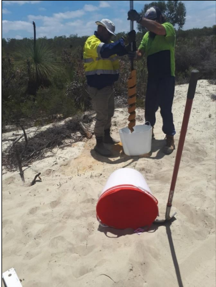
Figure 3: Hand auguring yellow sand at Arrowsmith
