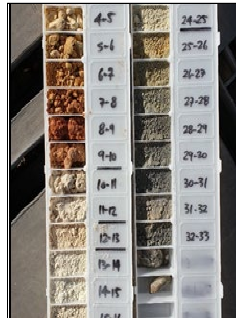
Figure 4: (above), shows drill hole GBAC069* which intersected 10m of light-white kaolinitic saprolite (10m -20m down-hole) beneath 10m of cover soil/calcrete, developed over micaceous granitic-gneiss basement.
