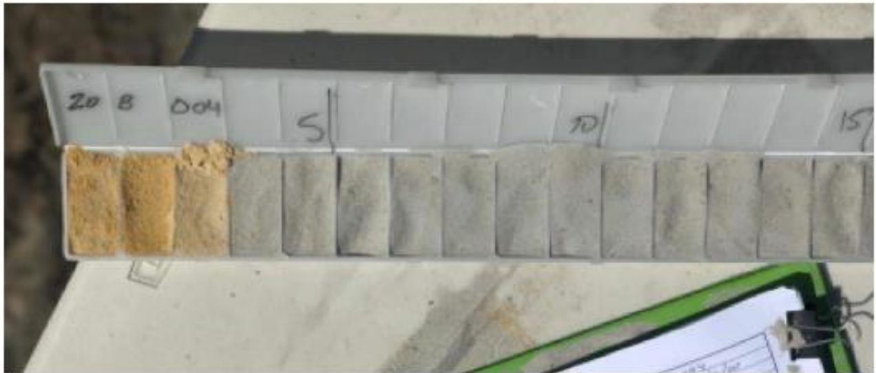
Figure 4 - >12m intersection of white sand separated into 1m intervals from the September 2020 Beharra drill program.
