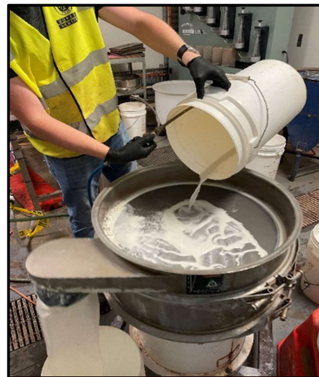
Figure 3: Wet sample screening for size fraction analysis of white kaolinitic saprolite clays from the Gibraltar Project South Australia.
