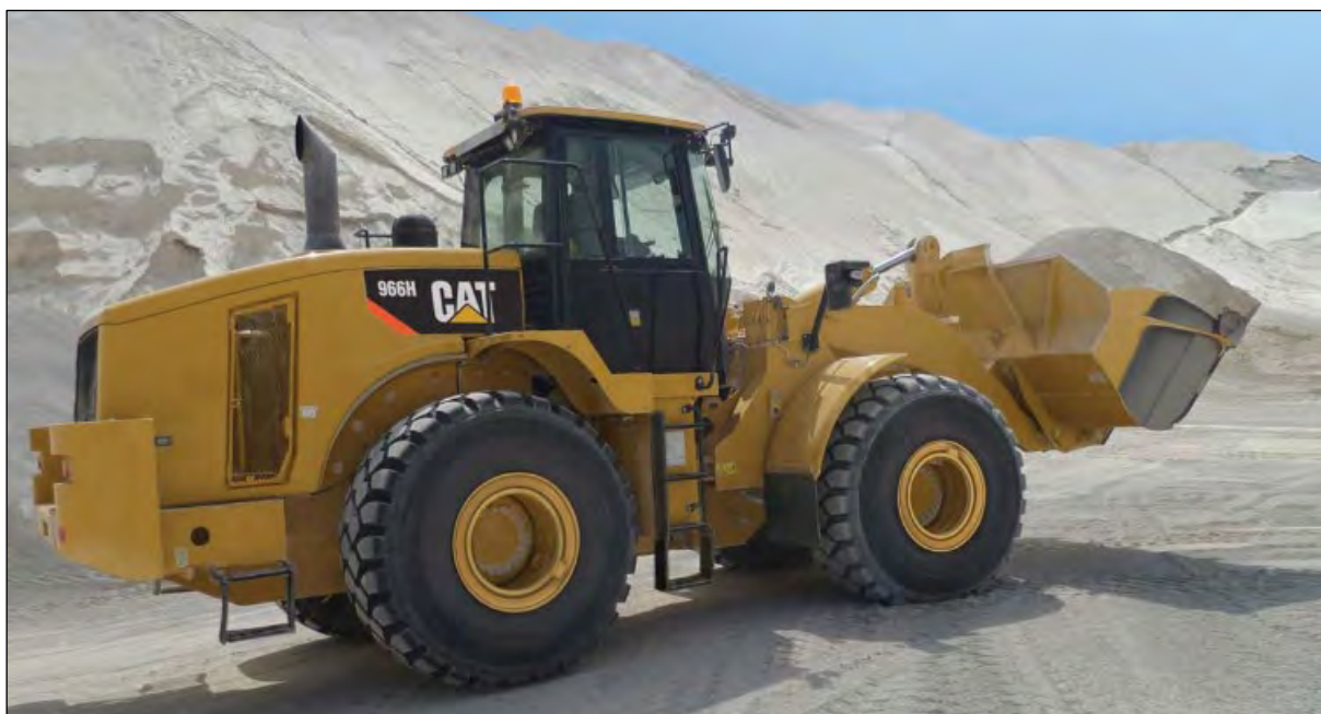
Figure 3.4 50-tonne operating weight FEL
