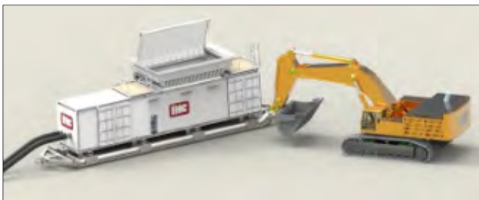
Figure 13.3 Alternative skid containerised unit
