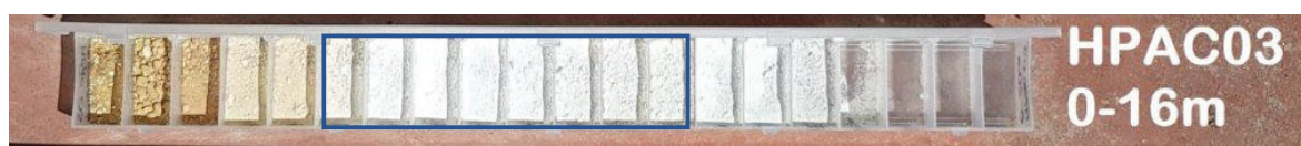
Figure 13 HPAC03: 8m @ 35.67% Al 2 O 3 , 0.46% Fe 2 O 3 , 0.11% K 2 O, 0.07% Na 2 O, 0.38% TiO 2 from 5m (assay on -45µm fraction)
