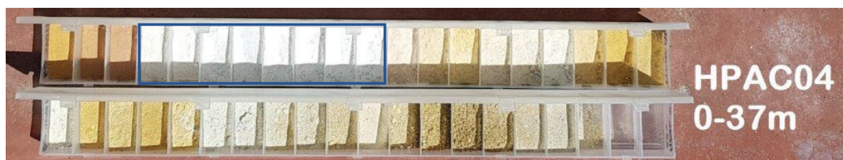
Figure 14 HPAC04: 8m @ 36.45% Al 2 O 3 , 0.42% Fe 2 O 3 , 0.25% K 2 O, 0.03% Na 2 O, 0.36% TiO 2 from 3m (assay on -45µm fraction)
