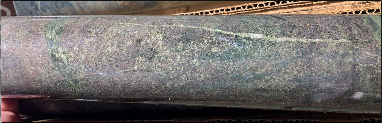
Figure 4 Strong copper mineralisation (chalcopyrite, yellow) in core from WT-21-04. (288.4m to 288.7m) The high-grade zone is approximately 10m in downhole length. Assays pending.
