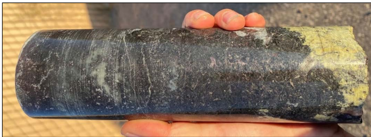
Figure 2 - WT-20-04, 186.4m down hole depth. Zone of semi-massive bornite and chalcocite within a broader zone of mineralisation of approximately 9.6m (visual estimate). HQ core size is approximately 30 cm in length.
